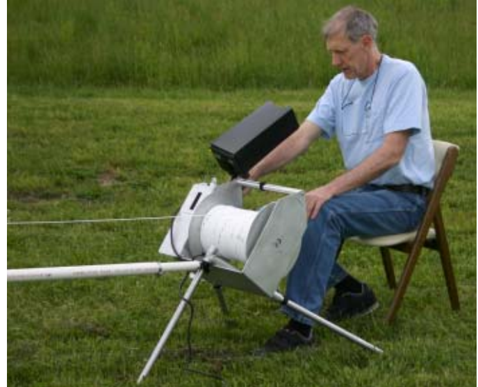
The Deluxe GeoVISION™ system in field use. Note the push pole attached to the front to provide additional stability in deep boreholes.
